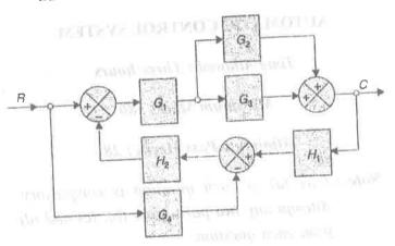
(d) Obtain the overall transfer function C/R from the signal flow graph shown in fig. using Mason Gain Formulae.
